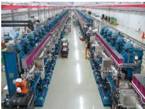
Fig. 1. New BL2 undulator line (left) installed in the SACLA undulator hall together with the existing BL3 (right).
