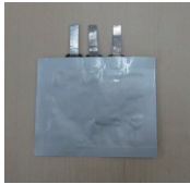
Conventional battery cell for X-ray measurement: thinner cell so that X-rays can be transmitted
