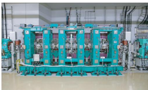
③The undulator produces X-rays (synchrotron radiation)
